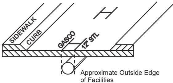
These examples indicate an operator's 12 in. facility. When a facility can be located or toned separately from other facilities of the same type, it is marked as a single facility.<sup>41/</sup>
