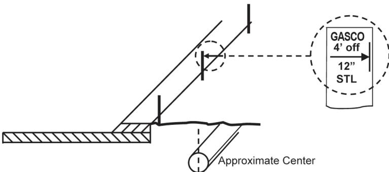
4. An operator's identifier (name, abbreviation, or initials) is placed at the beginning and at the end of the proposed work. In addition, subsequent operators using the same color mark their company identifier at all points where their facility crosses another operator's facility using the same color. Reduce the separation of excavation marks to a length that can reasonably be seen by the operator's locators when the terrain at an excavation site warrants.
