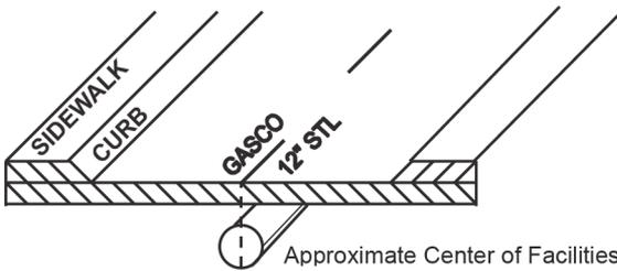
or 2) placing the marks over the approximate outside edges of the facility with a line connecting the two horizontal lines (in the form of an H) to indicate there is only one facility:
